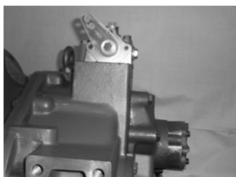
SHALLOW BOX PORT SIDE LEVER FORWARDS SUITS LH PROPELLER – AHEAD
