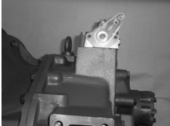
DEEP BOX PORT SIDE LEVER BACKWARDS SUITS LH PROPELLER – AHEAD
